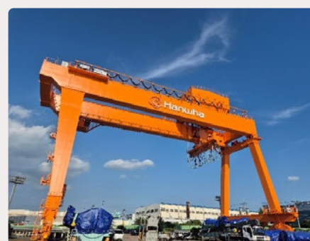
Gantry Crane 650ton
