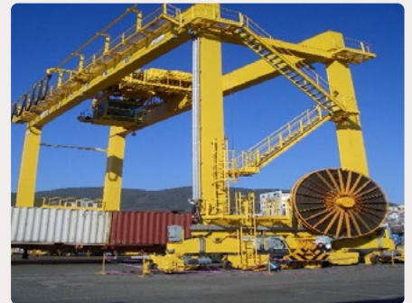
RMGC CY Yard Crane
